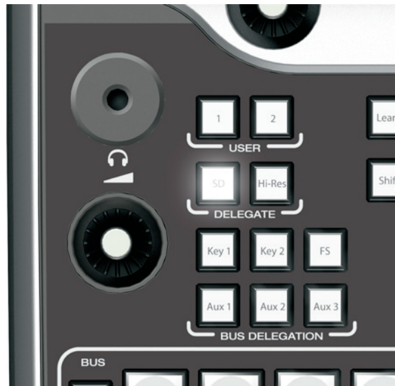
Figure 6 – Select the SD or the Hi-Res button in the delegation area to switch between SD mode and high-resolution mode
